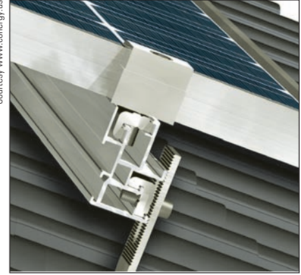
Almost all residential PV racks are “top-down,” meaning modules are easily installed from above. Typical examples (from L to R): IronRidge, Unirac, and Conergy. All show foot, rail, and clip.
